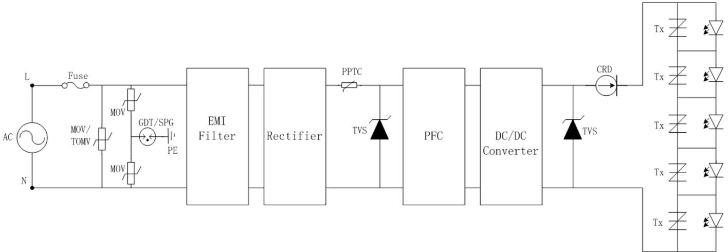
Figure 6: Overall protection design for LED drive circuit
