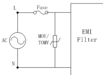
Figure 2: Differential protection mode of AC supply
