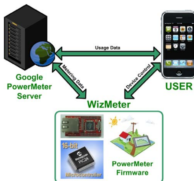
Fig. 1 EVB-PIC24 operation for PowerMeter
