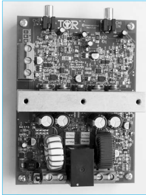
Figure 5: International Rectifier IRAUDAMPI demo board. Features 500W + 500W peak stereo power, efficiency 93% at 1 kHz and 100 watts. Voltage supply \pm 50 Volts (allowed \pm 25 to \pm 60 ). Compact size: 100 x 140 x 38 mm.
