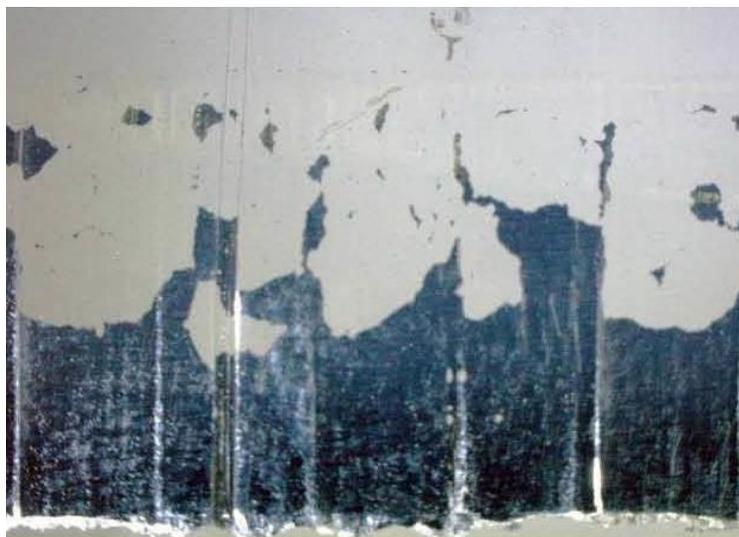
**Figure 2: Film metallization displaying significant corrosion.**
