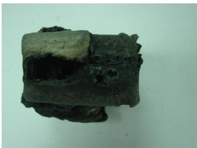
**Image 7: Image of a film capacitor which began to burn during an 85/85 test (THB test).**
