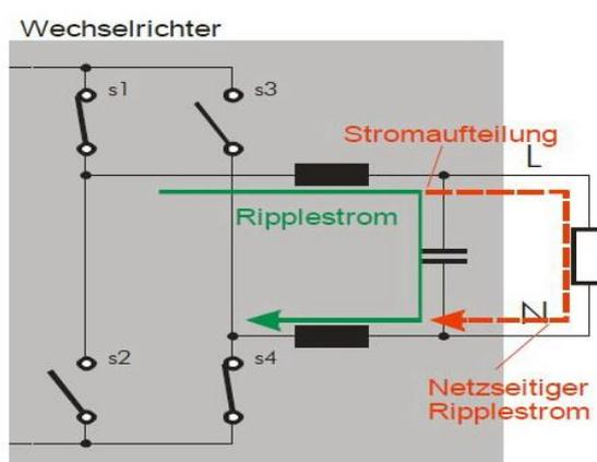
**Image 9: Ripple current distribution between electronic device using an X capacitor and the mains in a low impedance grid.**
